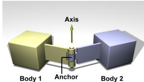
Figure 4.1: Hinge Joint ( [Smi06] )
